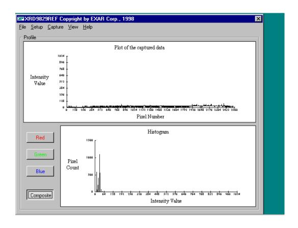
Figure 8. Black Target Scan After Global and Fine Adjust
